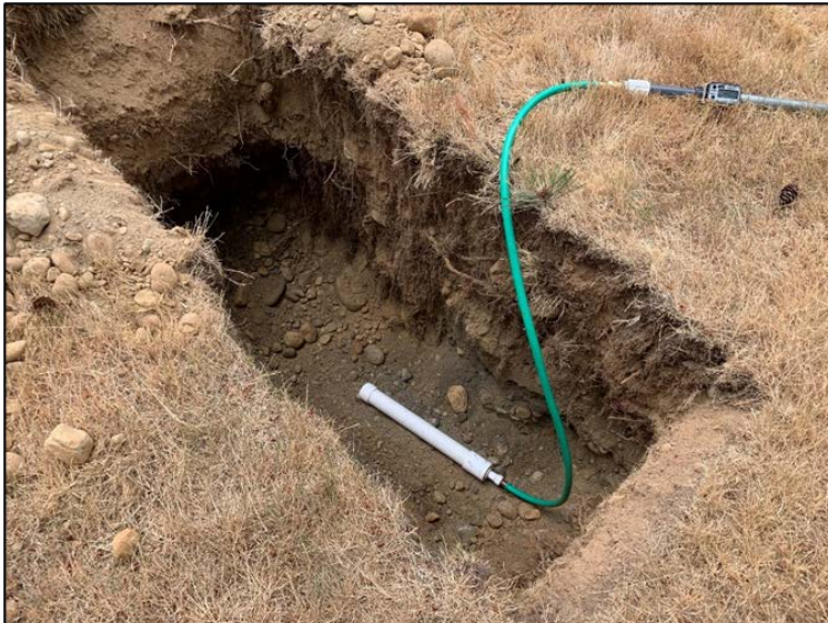
Plate 3: Typical infiltration testing setup.
